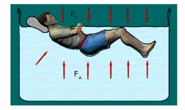
Fig. 4. An experimental model of dry immersion. When the body is immersed in water, the resulting force of hydrostatic pressure (Archimedean force,  $F_A$ ) balances the force of gravity ( $F_T$ ). However, the Archimedean force is distributed over the entire body surface. Because of that, the pressure on each point per unit body surface area is much lower than the support reaction force in the contact area in an upright, sitting, or prone position
