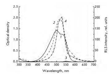
Fig. 1. Absorption (1, 2) and resonance light scattering (3, 4) spectra of a 25  $\mu$ M MC540 in distilled water (1, 3) solution and in 0.25 M NaCl solution (2, 4).
