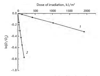
Fig. 5. Dose-response curves of photobleaching of a 25  $\mu$ M MC540 in distilled water (1) and in NaCl-containing (0.25 M) solutions (2). D and D<sub>0</sub> are the optical densities at 518 nm measured in irradiated and nonirradiated solutions, respectively.
