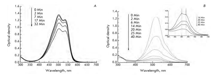
Fig. 4. Photobleaching of MC540 (25 µM) in distilled water (A) and in NaCl containing (0.25 M) solutions (B).
