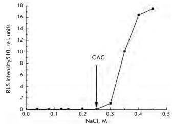
Fig. 2. Dependence of the RLS intensity at 510 nm in a 7.6  $\mu$ M MC540 solution on the NaCl concentration. An arrow indicates the critical aggregation concentration (CAC) of NaCl above which formation of MC540 aggregates occurs; the latter are detected by the RLS technique.
