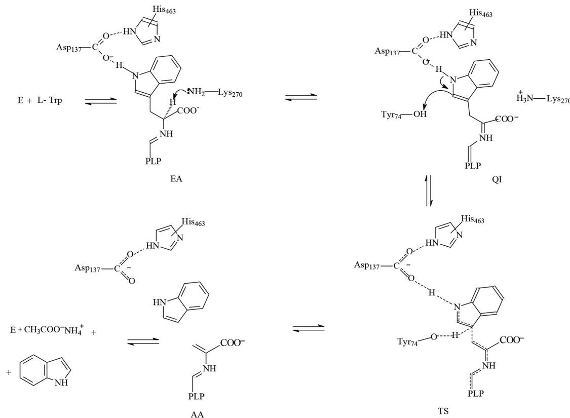
**Scheme** The principal mechanism of the reaction between TIL and L-tryptophan, which is consistent with [12–18]. E – internal aldimine; EA – external aldimine; QI – quinonoid intermediate; TS – transition state; and AA – aminoacrylate
