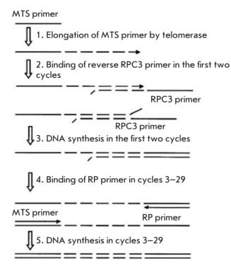
Fig. 4. "Two-primer" TRAP scheme [23, 24].
